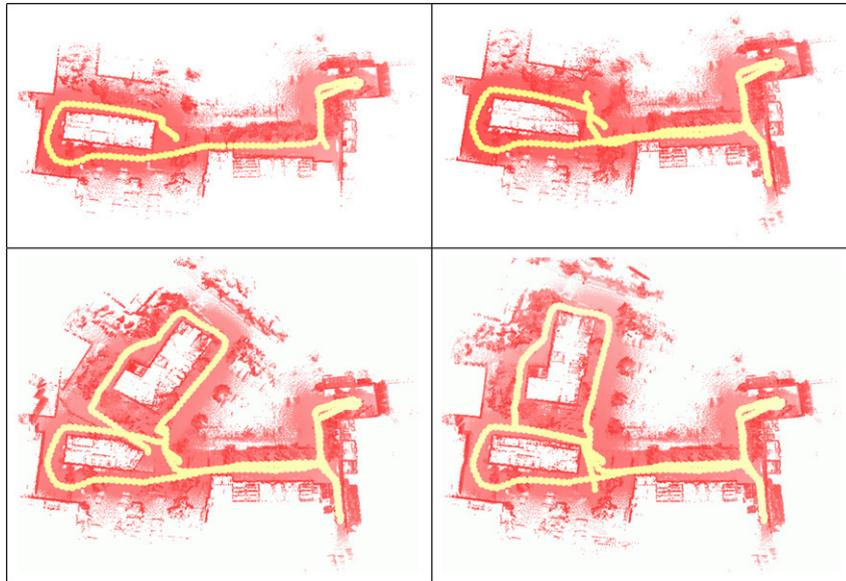
Fig. 6. LUM iterations at second, third and fourth closed loop. Top: second and third loop closing. Bottom: fourth loop closing after one iteration and after 20 iterations. Notice the merging of the robot path through graph recomputation in the fourth loop closing! (see Fig. 7 for the corresponding graphs, Fig. 8 for the resulting map).
